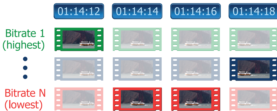
Figure 2 – Adaptive streaming technologies effectively ‘switch’ between bit rates by downloading segments of multiple outputs based on current conditions.
